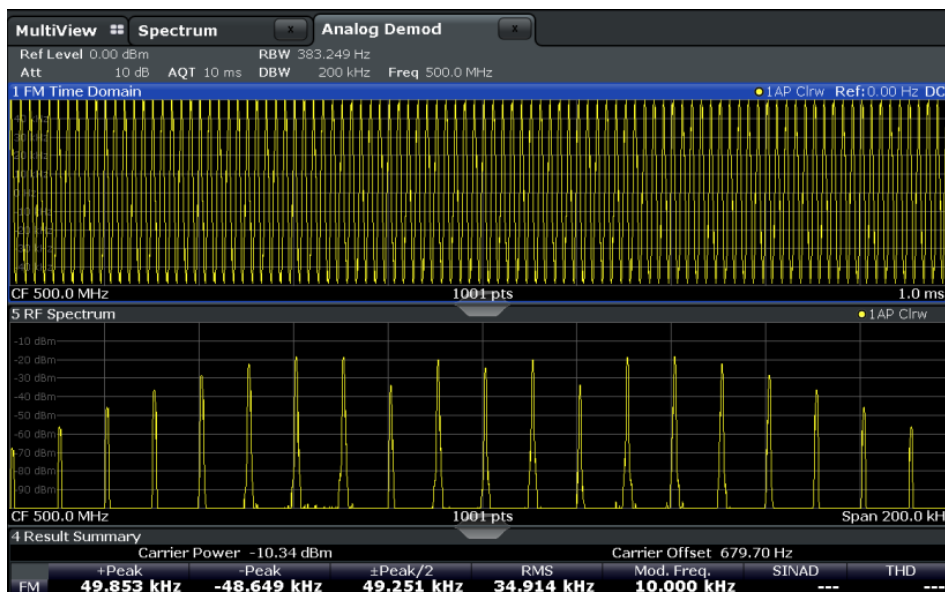
Fig. 9-5: RF spectrum with demodulation bandwidth = 200 kHz
